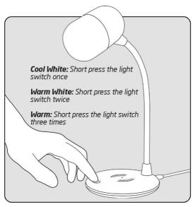
You can adjust the brightness whilst in any of the colour modes simply by holding down the light switch until you reach the desired level.
